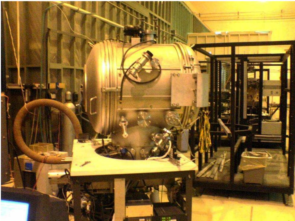
**Figure 31: Varian 0.76m x 1.0m vacuum chamber**
