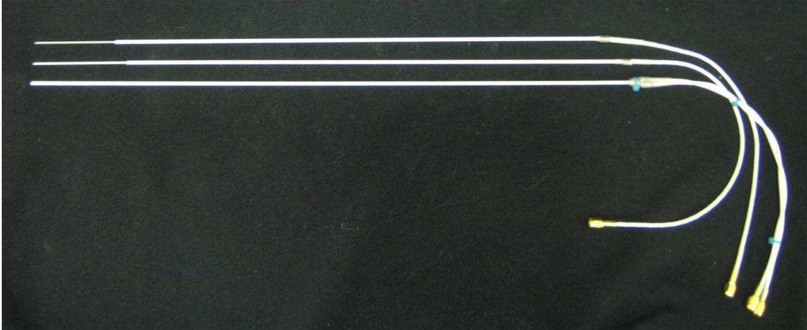
**Figure 12: Completed Langmuir probes of different types: A segmented Langmuir probe (Top), a standard Langmuir probe (Mid), and a double Langmuir probe (Bottom).**
